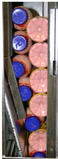
Front column properly loaded
