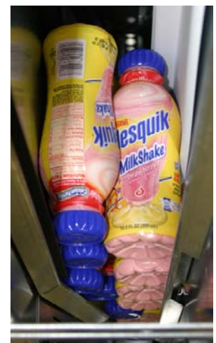
Front column properly loaded
