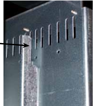
Right column wall, top, set in position 7
