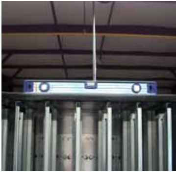
Leveling the front of the vender
