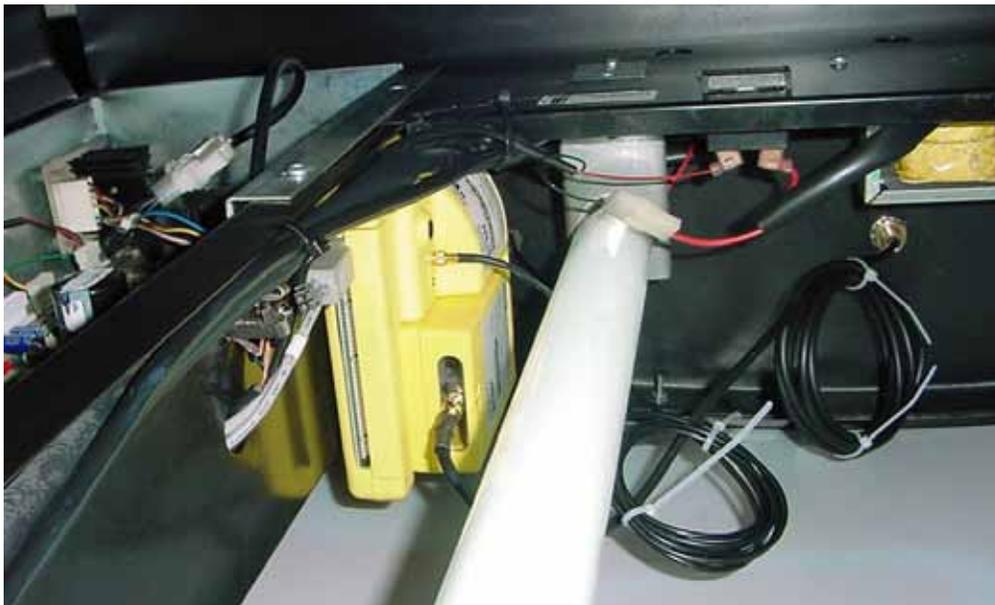
As shown here, the RDP unit should be mounted at the top of the door. Mount the antennas in the top of the door, with the taller antenna farthest away from the unit. Bundle and secure the antenna wiring. The antenna wiring should always be kept away from other wiring as much as possible.
