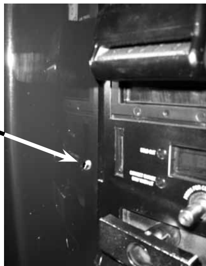
Figure 33. Use a 1/4" (6 mm) bit to drill two holes adjacent to the control panel. One of these holes is shown here.
