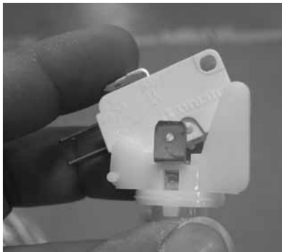
Figure 17. Insert the micro-switch into the switch holder.
