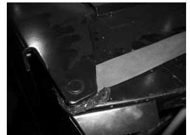
Figure 25. Trim the foam strip on an angle at the hinge on the left side.
