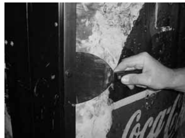
Figure 3. Removal of the Christmas trees. Slide the putty knife between the sign face and the trim, so as not to scratch the surface of the trim. Then, tap the handle of the putty knife to break off the head of the Christmas tree.
