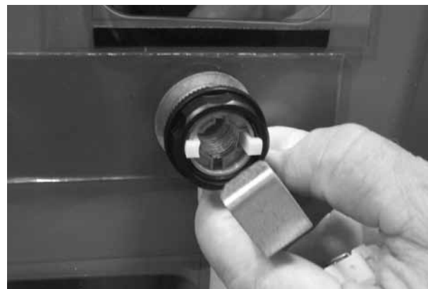
Figure 16. Install the washer on the shaft of the button, then install the lock nut.
