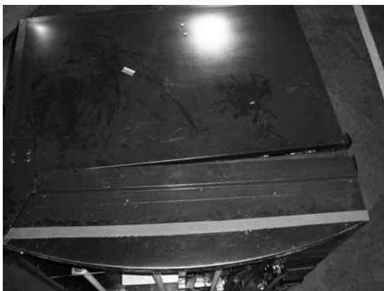
Figure 23. The foam strip should run straight across the width of the door as seen here.
