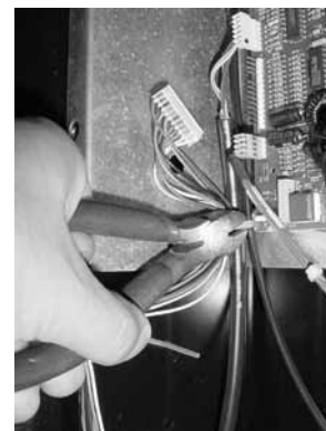
Figure 10. Cut any wire ties that secure the select switch harness in the vender.
