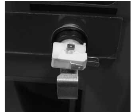
Figure 19. Finished button assembly.
