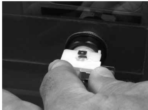
Figure 18. Insert the switch holder into the shaft until it snaps into place.
