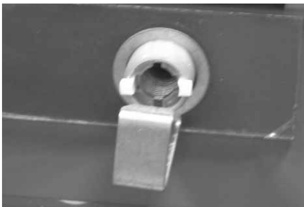
Figure 15. Switch retainer on button shaft.
