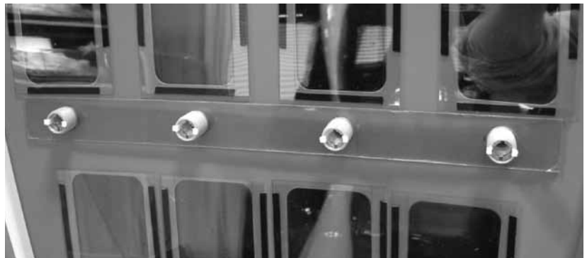
Figure 14. Install the button bar bracket as shown.
