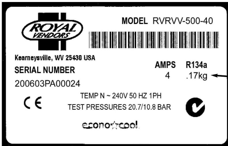
Place replacement decal over the incorrect R134a charge listed on the serial plate.
