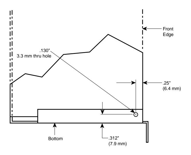
**Note:** Align template with front and bottom edges of housing prior to drilling. It may help to fold or cut the template.
