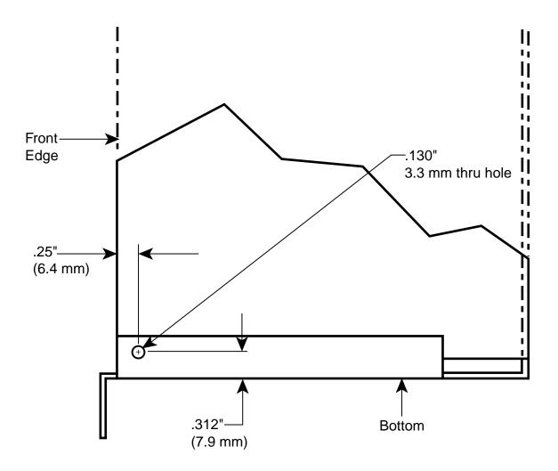
**Note:** Align template with front and bottom edges of housing prior to drilling. It may help to fold or cut the template.
