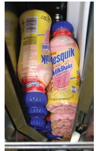
Front column properly loaded
