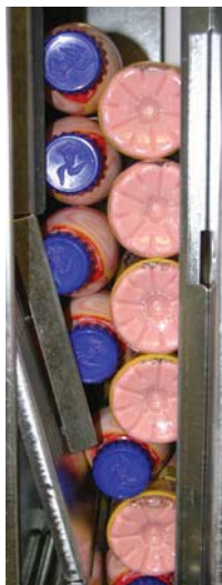
Front column properly loaded
