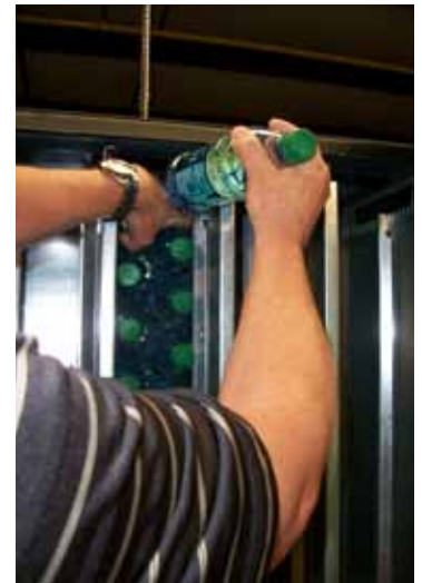
Overfilling the column. Note that this column is already full. Adding more product will compress the bottles, which causes vending problems, such as bridging.
